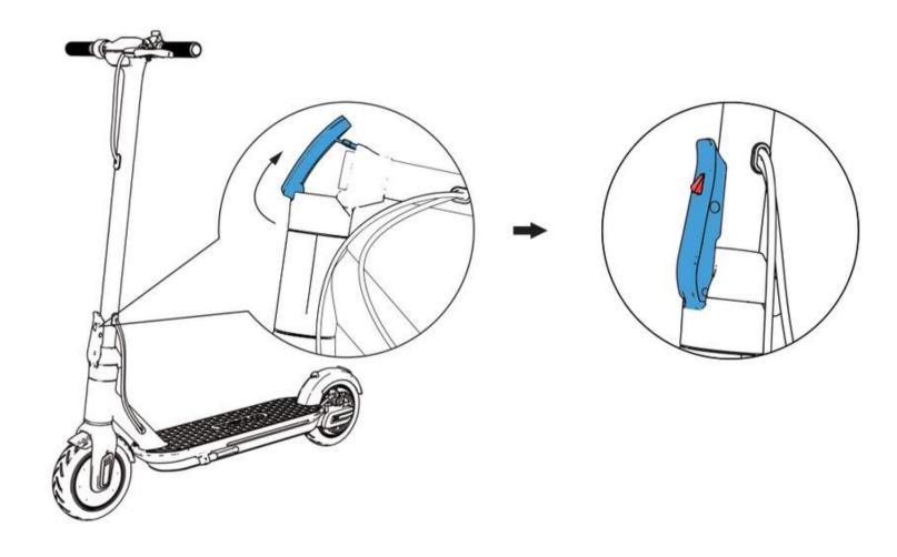
3. Fasten the scooter standpipe and fold out the kickstand.
