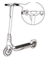
4. Install the handlebar to the standpipe.
