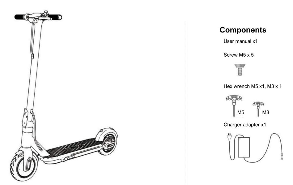
\*Please check carefully that the parts in the package are intact.
