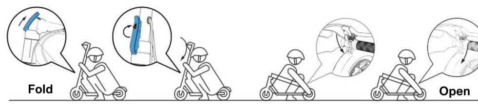
Put the safety-lock (the red part of the image) up whilst holding the steer tube. Then, open up the folding spanner (the blue part of the image) and aim it at the bell and fender hook. Next, buckle the belt with the back-fender.
