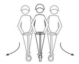
Solution Forbidden to rotate the handle strongly while driving with high speed.
