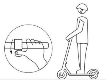
3. Once you have the electric scooter moving above 5km, put both feet on the deck and push the throttle to start the electric.
