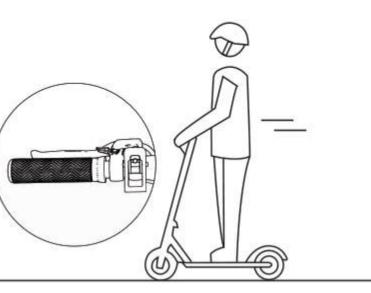
4. Releasing the throttle will slow you down gradually, with an automatic energy recover system coming in. For hard braking pull the lever on the left side.
