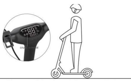
6. Keep to one speed for approximately 8 seconds to start the cruise control. When you release the throttle ,this then means the speed will remain unchanged. To cancel the cruise control, push the throttle or operate the brakes.
