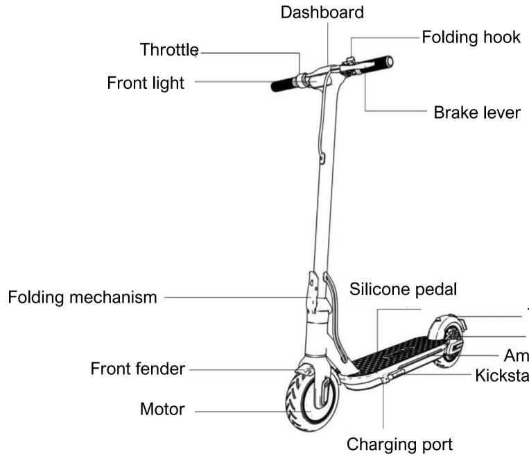
Tail lamp - Disc brake - Ambient light Kickstand
