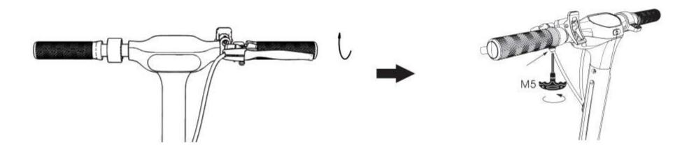
2. Hold the scooter upright, to ensure that the lock will not be affected, please keep the folding-spanner (the blue part of the image) at the bottom. Pull the folding-spanner to the top, then the scooter is completely locked.
