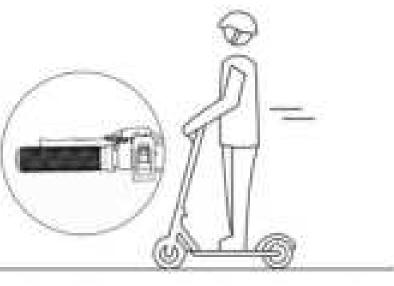
4. Releasing the throttle will slow you down gradually, For hard braking pull the lever on the left side.
