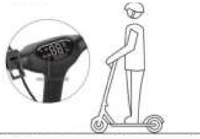
6. Keep to one speed for approximately 8 seconds to start the cruise control. When you release the throttle, this then means the speed will remain unchanged. To cancel the cruise control, push the throttle or operate the brakes.
