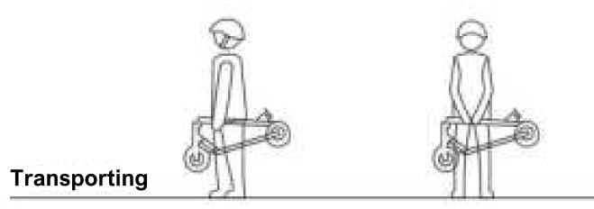
After the e-scooter has been folded successfully, use one hand or two to hold the folding-level to transit.
