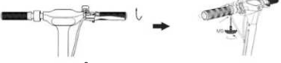
2. Hold the scooter upright, to ensure that the lock will not be affected, please keep the folding-spanner (the blue part of the image) at the bottom. Pull the folding-spanner to the top, then the scooter is completely locked.
